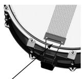
Distance: distance of between 5-7mm to the edge of the drum rim.
